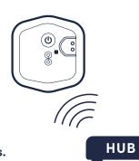
confirm blobutton activation by pressing the button and verifying that the light blinks GREEN 4 TIMES. If the blink pattern is different or the light does not blink, refer to the Indicator
