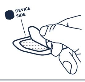
Place the **BIOBUTTON** on the exposed adhesive. Turn the device over and remove remaining adhesive backing.
