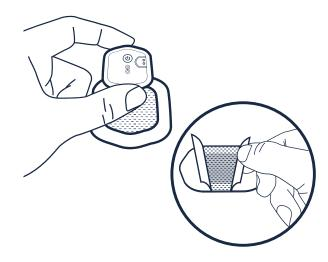
ADHERE the BioButton Rechargeable device to upper left chest placement area near the sternum. Apply pressure for 15 SECONDS.
